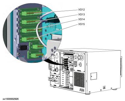
The connectors are internally connected with the I/O unit (DSQC 652).
