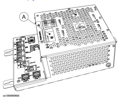
A Assembled expansion board for fieldbus adapters, without adapter.
