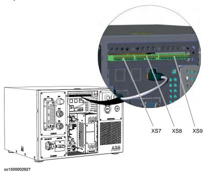
These connectors is internally connected with safety board.
