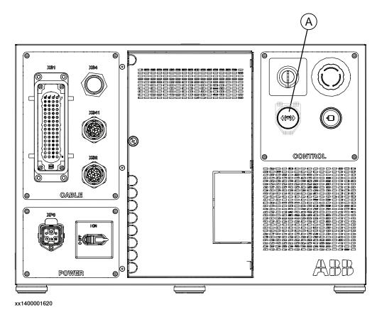
A Brake release button (under the cover) for IRB 120.
